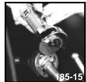
185-15 Pneumatic Cut Off Tool: Joint Removal When Internal Circlips Lock Joint On Shaft
