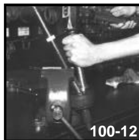
100-12 Inner Race Driver: For Removal of Joints With Frozen Internal Snap Rings
